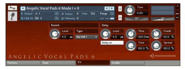
On the FX page, you can apply a delay effect and a high-quality convolution reverb. From left to right, the controls are as follows:
